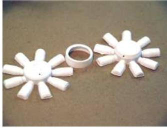
Assemble the motor halves by dropping the alignment ring in one of the halves. Place the other half in place with out cement. Find the cylinders with a dimple near it's base on the engine case. These
