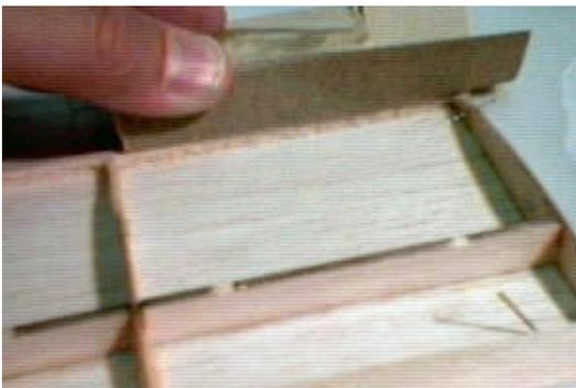
Sand 1/8 x 1/4 stock at front of aileron bays until it is flush with, and matches the angle of the ribs.
