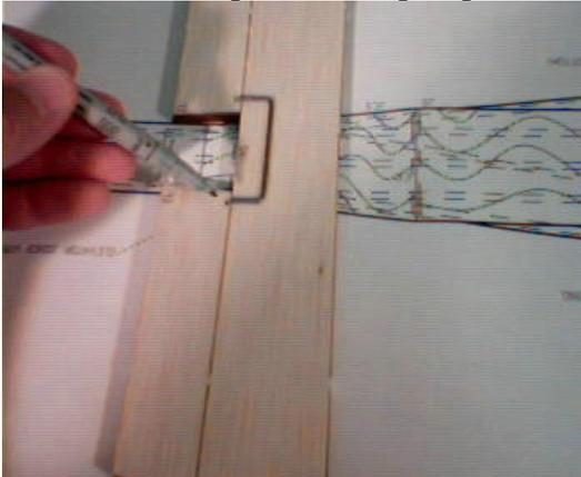
Lay **HS** and **ELs** in place the plan, and mark the locations for the joiner wire holes to be drilled in the elevators. Also mark the positions for the hinges at this point. 2 CYA hinges per side are recommended.
