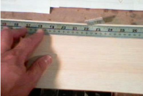
Run medium CYA along the straight edge of this sheeting, and glue it to the back of the leading edge, so that it is touching all of the ribs. Use a straight pin over each rib to ensure positioning. Fill any gaps with a gap filling glue that can be sanded, such as PICA Gluit.
