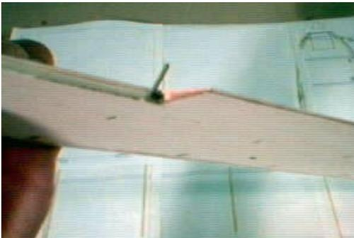
Fill gap between sheeting behind aileron torque rod, at inboard end of aileron bay with scrap balsa.
