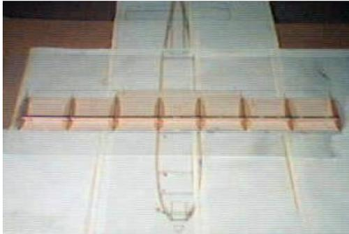
Glue 1/8 x 1/4 balsa stock to rear of outboard ribs, and flush with end of sheeting to form front of aileron bay. Butt glue the inboard end to **W1**. Repeat for other side.
