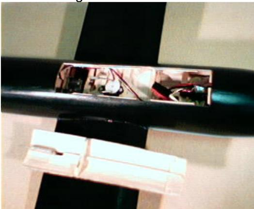
Cut hatches on top and bottom of fuselage, as shown on plans. Use scrap 1/16 balsa to form a flange on the inside of all sides of the bottom one, and the front and sides of the top one.
