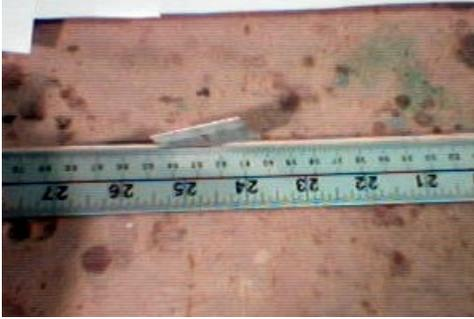
Check that 1/4 x 1/2 stock for leading edge is straight. If it has developed a warp along the 1/2" axis, used a straight edge to cut one edge completely straight. Ensure that the piece is not less than 3/8 high at any point.
