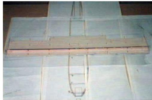
The ribs are then fitted to both the **SPAR** and the sheeting, again using the provided slots and tabs to ensure alignment. Note that there are now more ribs. **W1**'s go in the two most inboard positions, and **W2**'s go in the outboard positions. When all parts are in place, and the front of the ribs line up exactly with the front of the **BOTTOM WING SHEETING**, glue everything together using thin CYA, followed by medium CYA to form a fillet.
