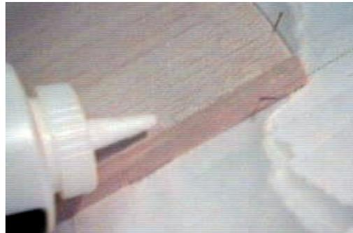
When glue is dry, carefully roll sheeting down on ribs, until aileron torque rods poke up through sheeting. Lift it back up, and cut 1/4 wide by 1/2 long slots around the holes made by the torque rods.
