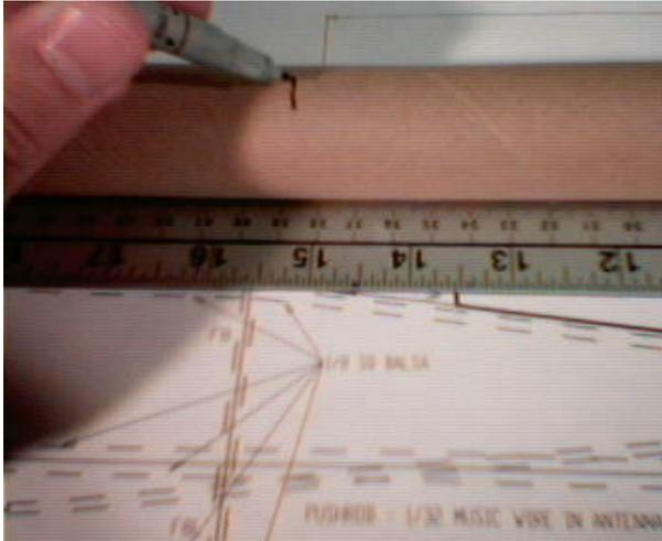
Measure 15” from one end of tube. This will be the rear of the rear former. Using plans, mark the position of the rear of the front former, as well.
