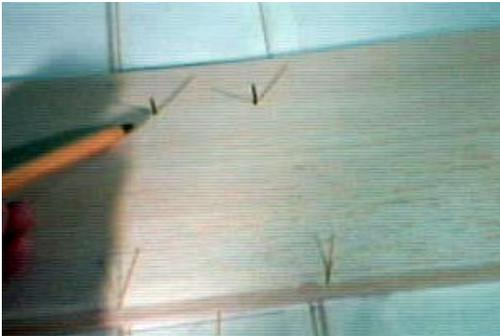
Completed slots for aileron torque rods.
