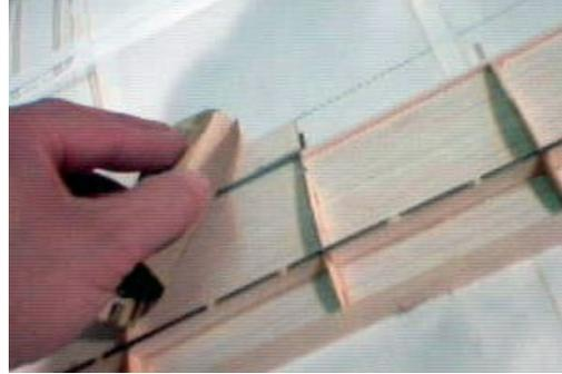
Using a straight edge and a single-edged razor, ensure that one edge of the 1/16" x 6" balsa sheeting is completely straight.
