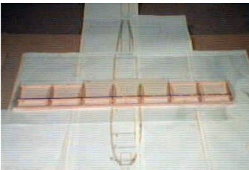
Glue leading edge in place, with straight side down on the building board. Go over each joint again to form fillets.
