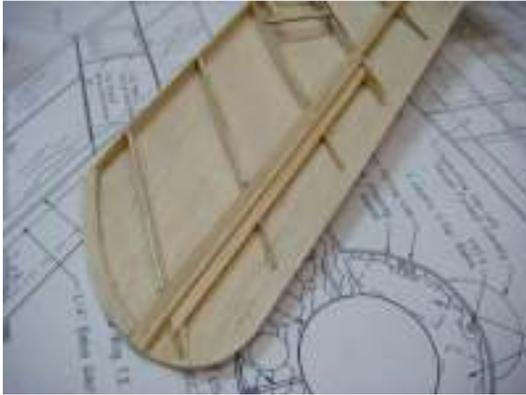
Mark the location for the aileron ribs using the marks on the plans and the angle gauge. Sand the 1/4" balsa aileron L.E. as shown on the plans. Glue the aileron L.E. to the top sheeting followed by the aileron ribs. Use pin holes to mark the location of the aileron. Plane the sub-leading edge flush with the ribs.
