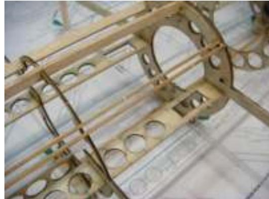
Glue the hatch formers to the top stringer using 1/64" plywood to space them from F2 and F4. Glue the H1 hatch edges in place. There should be an 1/8" gap between these pieces. Slip wax paper between the hatch formers and F2 and F4.
