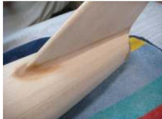
Apply a small fillet around the root of the wing, the fin, and stab. Final sand the airframe and prepare it for finishing.
