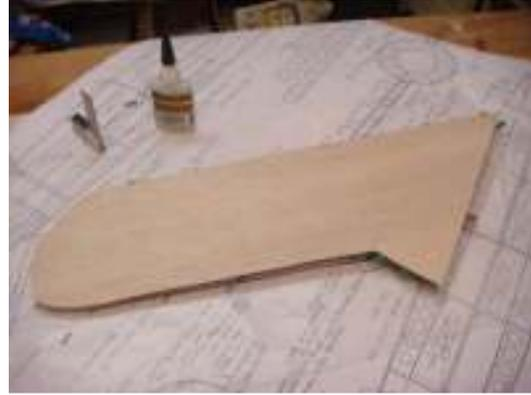
Remove the wing assembly from the board. Use pinholes to locate R2, R4, and R5 for the wing-fences.
