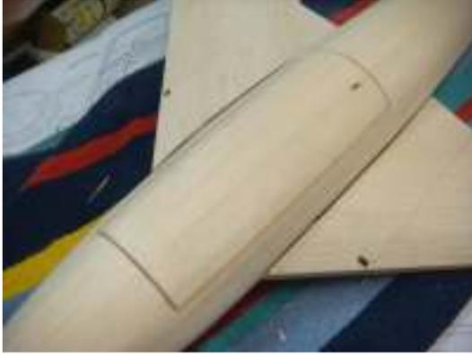
Glue a piece of 1/16" basswood to the H1's on the hatch and in the fuselage. Replace the hatch and sand the basswood edges flush with the planking. Trim the canopy to fit the hatch. It is glued in place after covering.
