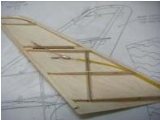
Install the elevator flex cable as shown on the plans. Remove the building tabs from the ribs and sheet the other side. Cut an opening in the sheeting between V3 and V4. Glue the stab in place, making sure it is square to the fin. Temporarily hinge the rudder and glue the control horn in place.
