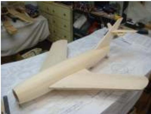
Slide each wing on to the spar and mark the wing sheeting with the shape of the fuselage. Trim the sheeting for a tight fit to the fuselage. R1 should touch the fuselage at F4. When satisfied with the fit, apply 30 minute epoxy and slide the wings in place. Jig the fuselage over the plans and pin the wing tip jigs in place. Double check the alignment and let it cure overnight.
