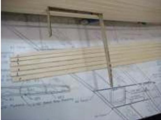
Use the planking template on the plans to cut 3/32" balsa planks. This will help reduce the amount of cutting and fitting. Slightly bevel the edges of each plank before gluing it in place. I've found that using sandable glue along the edges and CA to glue them to the formers makes quick work of this task. Plank the top of the fuselage as far as you can down each side.
