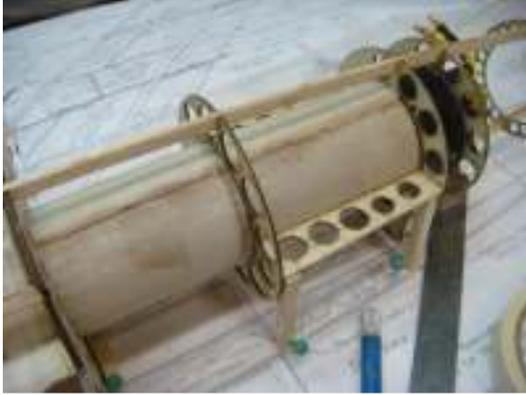
With full inlet ducting, there are considerable forces trying to collapse it during flight. Ensure that the duct material is solid and has no cracks in it and that it is securely glued to all formers. Cut the front and rear ducts from 1/64" plywood. The edges of the ducts overlap 1/4" and are beveled to provide a smooth duct.
