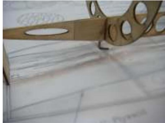
Bend the tow hook from 1/16" music wire and epoxy it in F12. Glue 1/64" plywood scraps to trap the tow hook in place. Complete the fuselage planking and sand the fuselage smooth. Cut holes to match the aileron servo lead holes in the wing root ribs and to clear the spar box.
