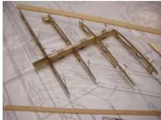
Glue the balsa spar box top and bottom (SB1) to the plywood spar box sides (SB2). Use two layers of scrap 1/16" plywood between the sides to ensure the spar will fit. Position R2 on the spar box and glue it in place up against the tabs. Slide R1 and R3 on to the spar box and glue in place. Glue the outer spar box top (SB3) and bottom (SB4) in place. Sand the outboard end of the spar box to match the L.E. Sand the front of each rib to match the angle of the L.E. (make right and left hand ribs).
