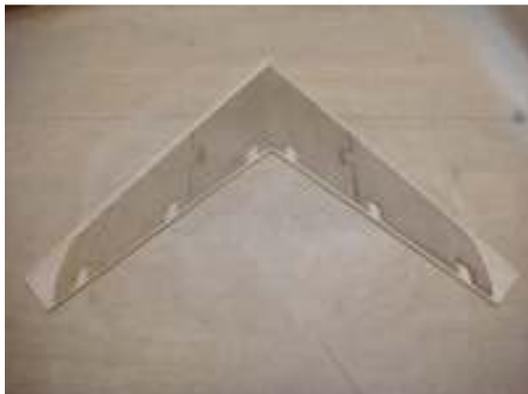
The stab and elevator are 3/32" balsa laminated around a central core of 1/64" plywood. The grain of the balsa should run parallel to the trailing edge of the
