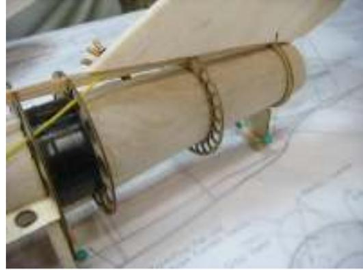
Use the template on the plans and cut and install the outlet duct. Make sure F8 and F9 are aligned and square to the board.
