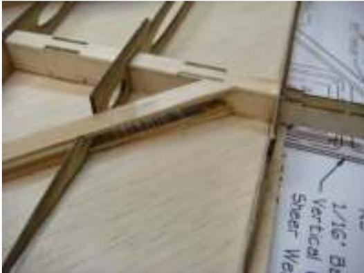
Glue R2A in place making sure it is level with the board. Glue the 1/16" balsa T.E. in place and sand the top to match the rear spars. Glue the 1/16" basswood sub-leading edge and plane/sand it flush with the ribs. Note there is a slight bend in the L.E. at R4 and it should taper slightly outboard of R7. Glue the top sheeting in place, and trim it flush with the L.E.
