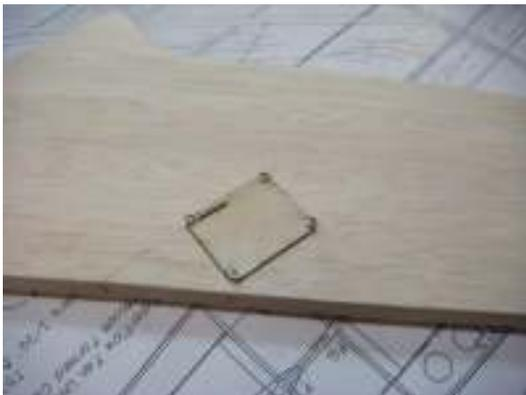
Glue the 1/16" balsa bottom sheeting in place. Use a pin to locate the servo hatch mounting holes. Use the 1/16" plywood servo hatch as a template to remove the bottom sheeting. The aileron servo is mounted to the hatch. Glue the 3/16" balsa L.E. in place and sand to shape. Locate the edges of the aileron and cut if
